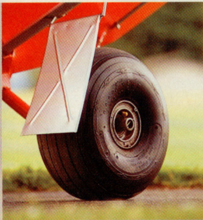
Mud guards (above left) prevent the main tires from slinging debris into the propeller disc. Ram air pressure pushes against the spring-loaded exterior plate of the safety meter (above center) and registers safe airspeed (the white band) or dangerous speeds (the red bands) on the instrument panel (above right).
